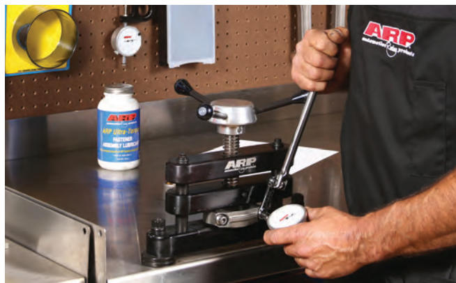
A rod bolt stretch gauge is one of the most important tools a serious engine builder can own. It's valuable in properly setting up a rod for resizing, obtaining the proper clamp load when installed. See page 172 for more information.
